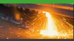
POMETON FERTAG iron powder is an essential element for the flame cutting process. Its ability to provide heat and raise the temperature of the flame, permits fast, deep and precise cuts with substantial time and cost savings.
