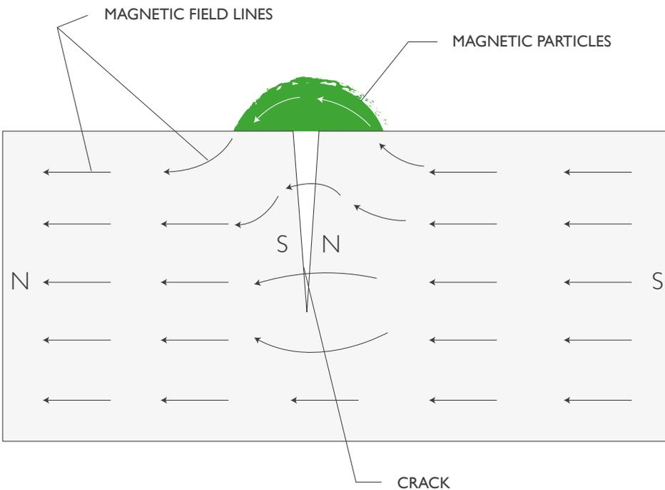
With the use of Ferilev powders, supplied also in titanium white color, it is possible to detect the dispersion of magnetic flux at the cracks.
