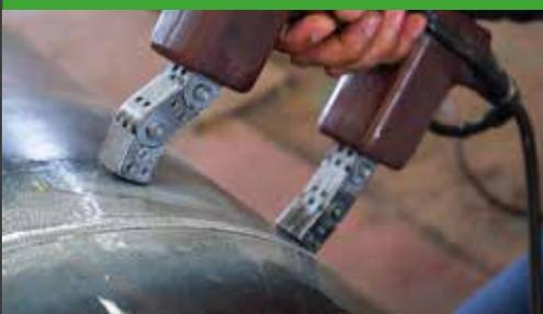
Thanks to their magnetic behaviour **POMETON FERILEV** iron powder is ideal in a number of magnetic applications, like non-destructive magnetic tests (i.e. on welding and casting discontinuity). This process permits to identify possible cracks or defects without damage the component.
