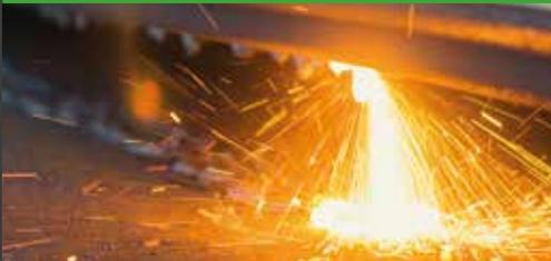
**POMETON FERTAG** iron powder is an essential element for the flame cutting process. Its ability to provide heat and raise the temperature of the flame, permits fast, deep and precise cuts with substantial time and cost savings.
